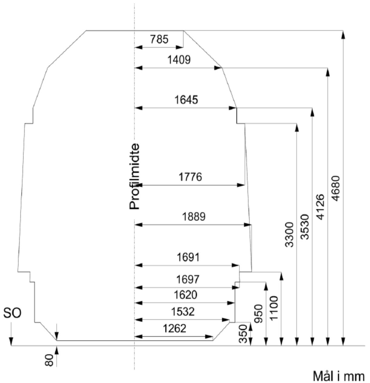
Kinematic reference line DE3, V > 200 km/h
